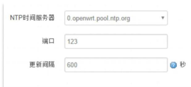
The screenshot shows three configuration fields for NTP. The first is 'NTP时间服务器' (NTP Time Server) with a dropdown menu showing '0.openwrt.pool.ntp.org'. The second is '端口' (Port) with a text input box containing '123'. The third is '更新间隔' (Update Interval) with a text input box containing '600' and a blue help icon with the unit '秒' (seconds).
